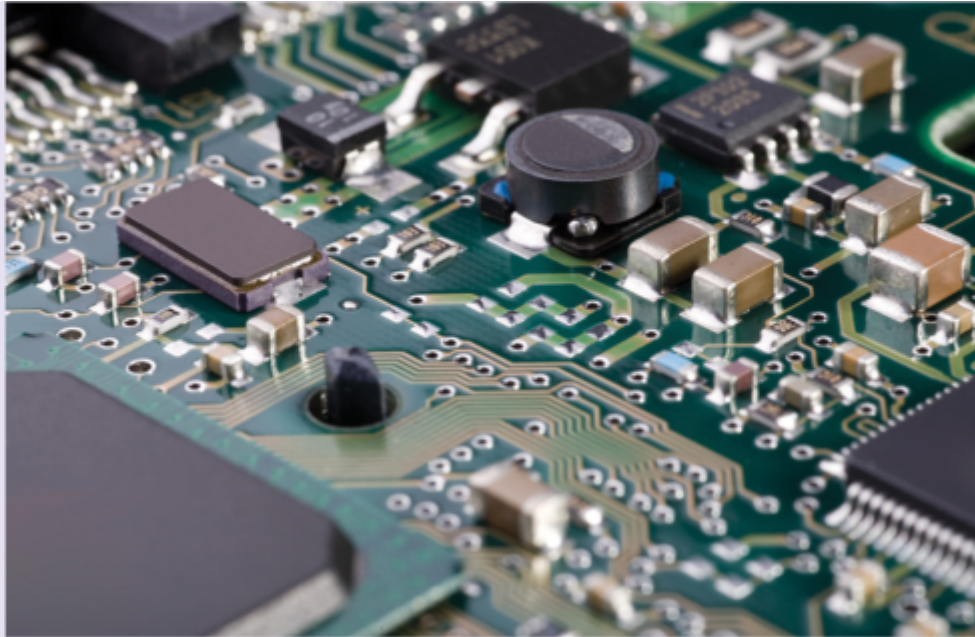
Figure 9.1: A complex electronic circuit – this is the circuit board that controls a computer’s hard drive.
