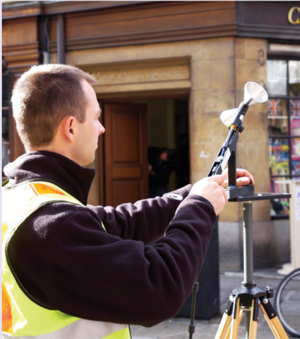
Figure 22.1: Mobile phone masts produce weak electric fields – this scientist is using a small antenna to detect and measure the field of a nearby mast to ensure that it is within safe limits.
