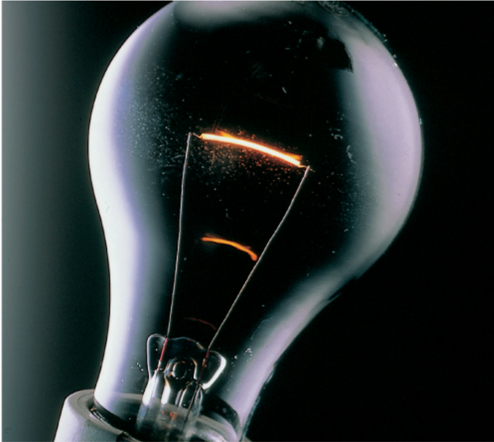
Figure 10.3: The metal filament in a lamp glows as the current passes through it. It also feels warm. This shows that the lamp produces both heat and light.
