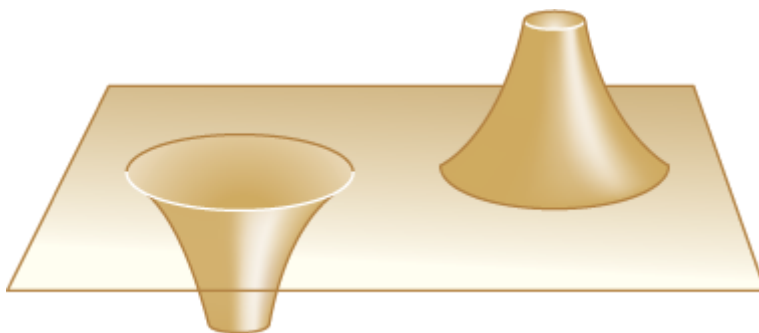
Figure 22.12: A 'potential well' near a negative charge, and a 'potential hill' near a positive charge.
