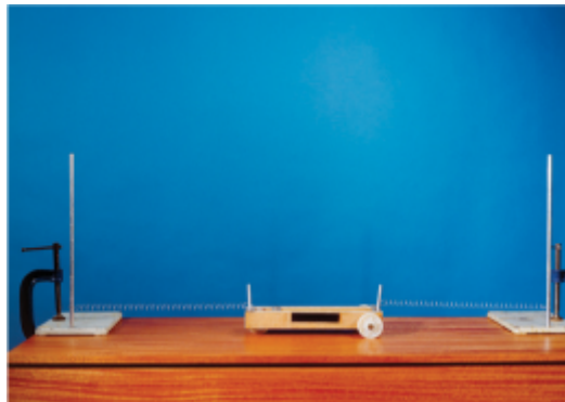
Figure 18.3: A trolley tethered between springs will oscillate freely from side to side.
