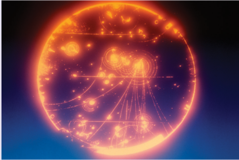
Figure 25.1: A bubble chamber image of the tracks of sub-atomic particles. The tracks curve because the charged particles are affected by the presence of a magnetic field.
