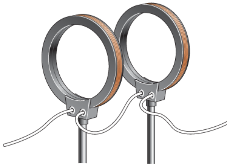
Figure 25.10: A pair of Helmholtz coils is used to give a uniform magnetic field.
