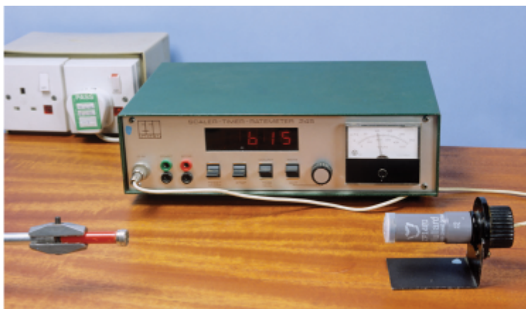
Figure 29.7: The time constant of this ratemeter can be adjusted to smooth out rapid fluctuations in the count rate.
