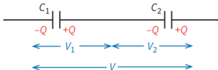
Figure 23.13: Capacitors connected in series store the same charge, but they have different p.d.s across them.
