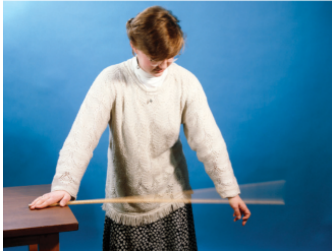
Figure 18.2: A ruler vibrating freely at its natural frequency.
